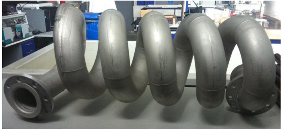
Figure 1c: The prototype of Spiral separator SaoxFuge DN100
