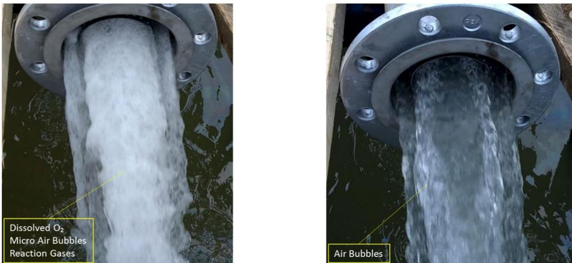
Fig. 6 Left OxTube aerated water flow and right non OxTube aerated water flow. OxTube aeration creates high concentration of dissolved O<sub>2</sub>, immediate reaction and huge amount of bubbles of 0.1 mm diameter in average. The surface tension and viscosity of the liquid is reduced significantly.
